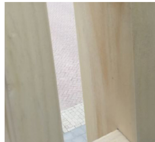
8.5 Reddish brown staining
