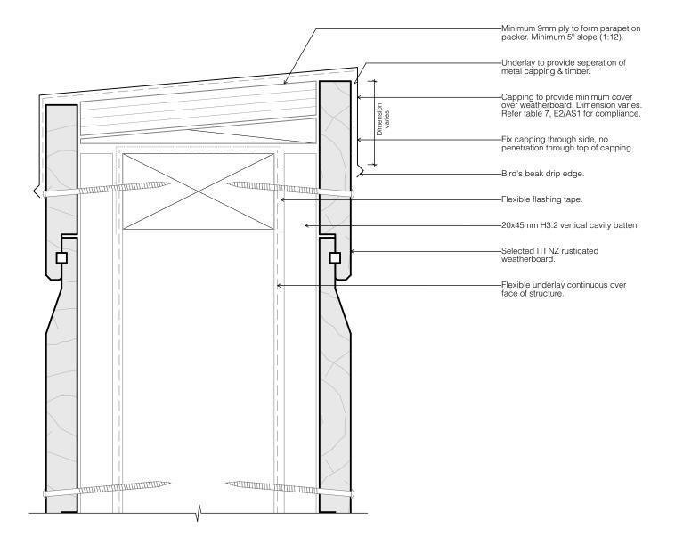
DETAIL 13.23 - 802 PARAPET - INTERSECTION WITH WALL
