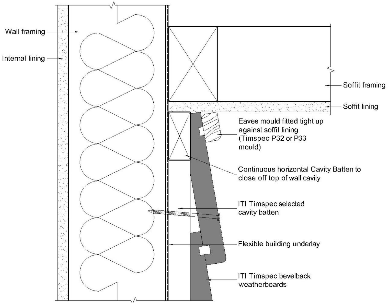
**FIGURE 13. 16 BC 602 ROOF/ WALL TOP PLATE – NO SOFFIT**
