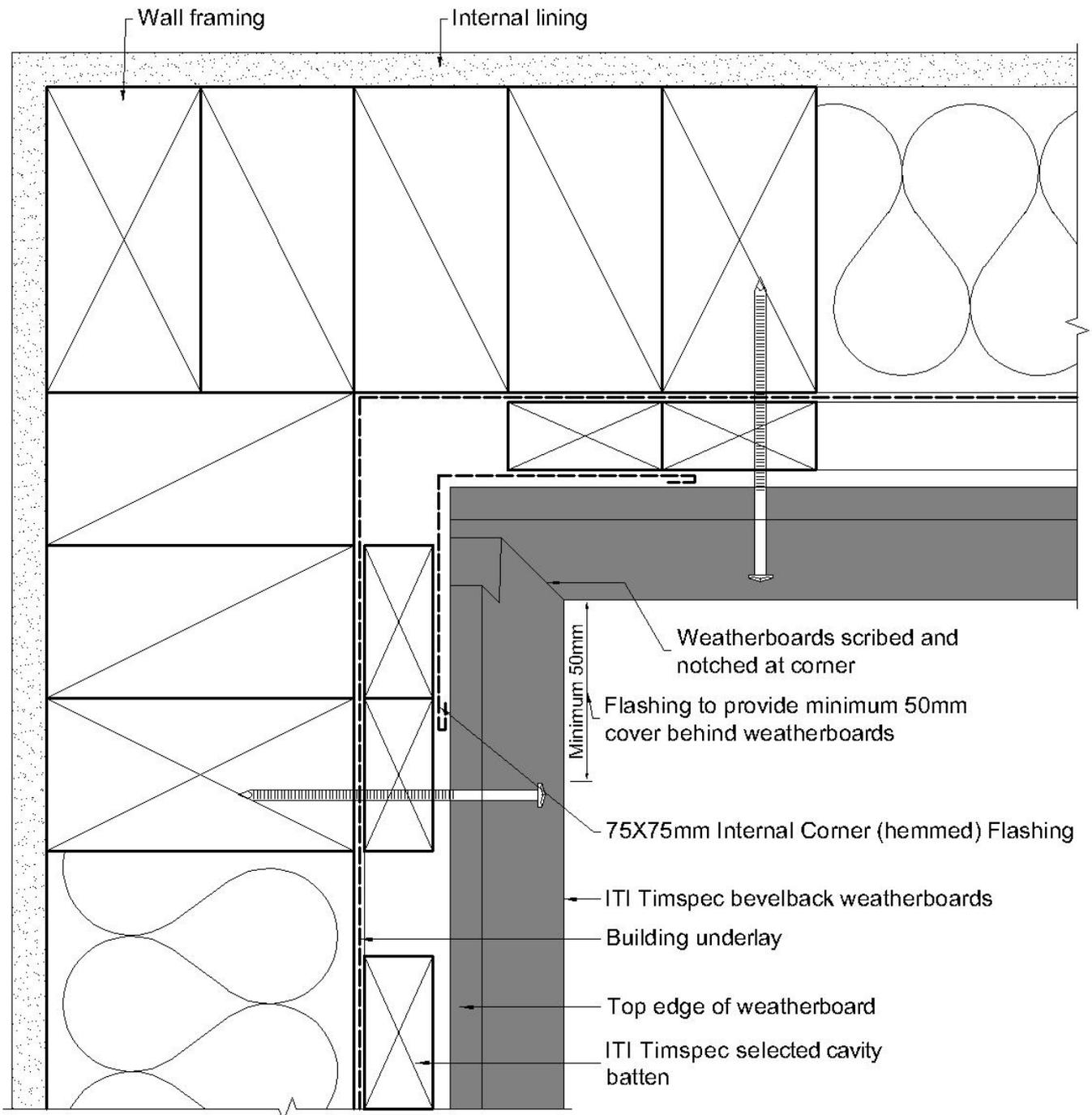
**FIGURE 13. 7 BC 302 INTERNAL CORNER MOULDING**
