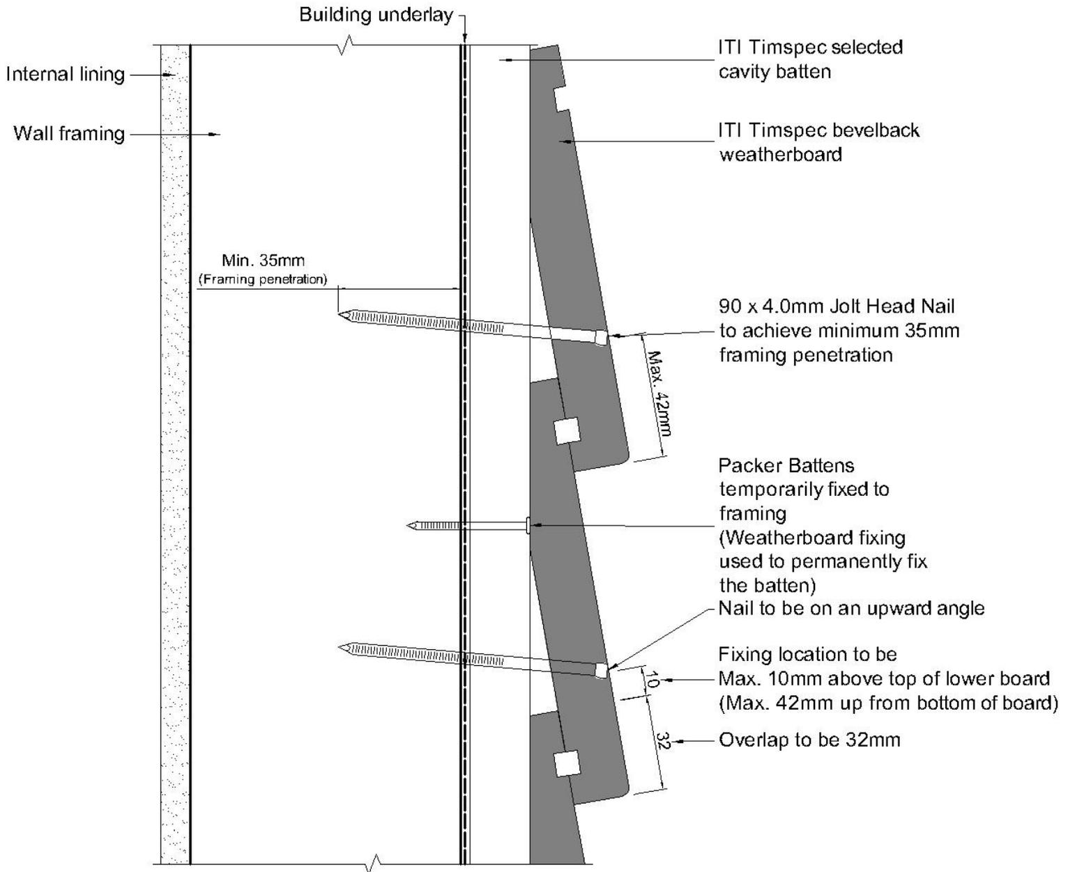
**FIGURE 13. 2 BC 108 STAIN FINISH WITH STANDARD CAVITY FIX**
