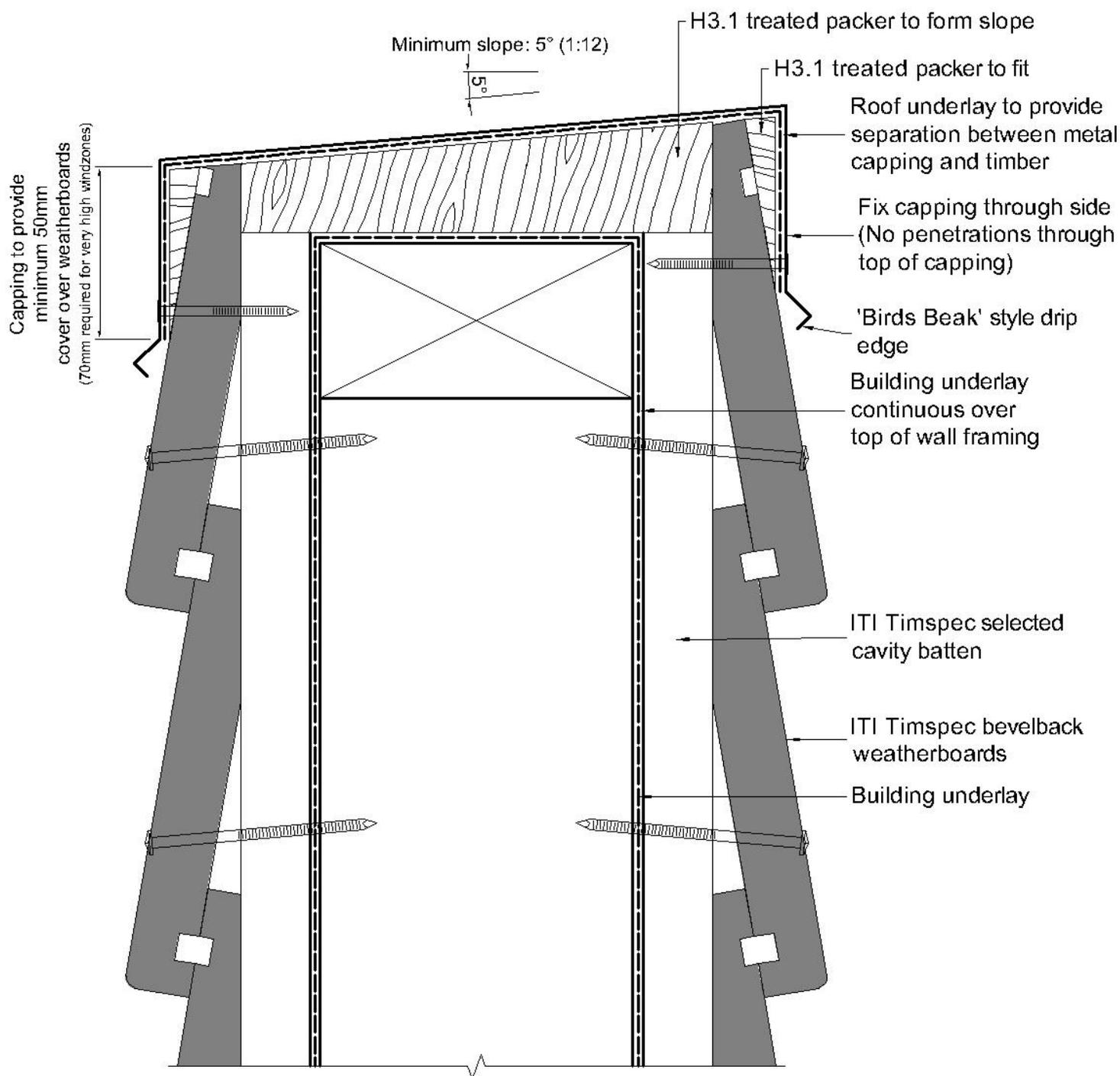
**FIGURE 13. 18 BC 702 BALUSTRADE INTERSECTION WITH THE WALL**
