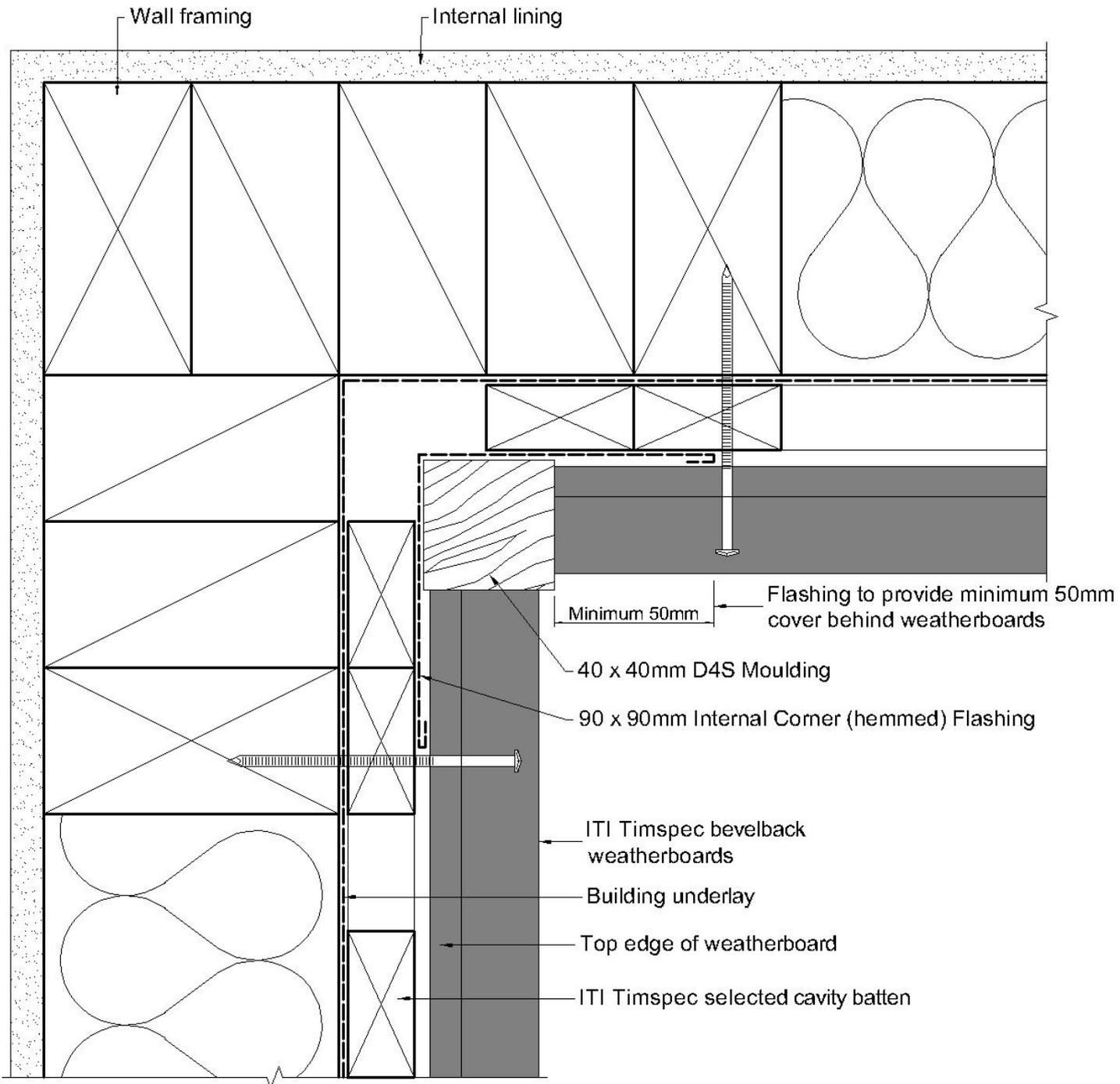
**FIGURE 13. 8 BC 401 INTER-STOREY CAVITY JUNCTION**
