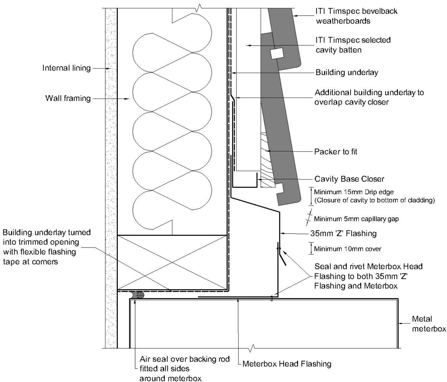
**FIGURE 13. 20 BC 802 METER BOX JAMB**
