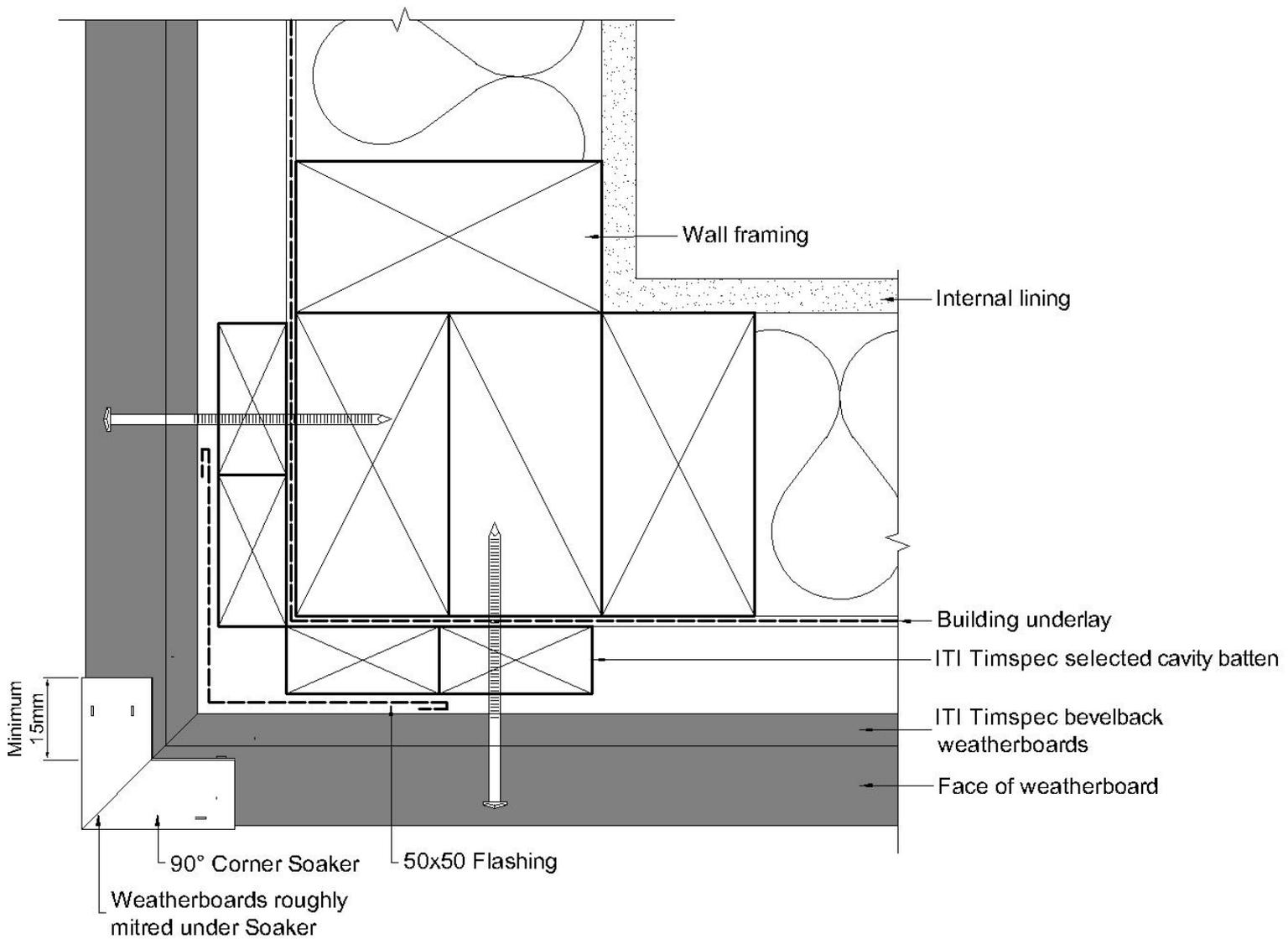
**FIGURE 13. 12 BC 501 BASE, TIMBER FLOOR**
