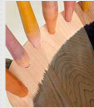
Vinegar with rusty metal in it brought out the tannins, highlighting grain pattern and texture. Fruit dyes coloured the spindles
