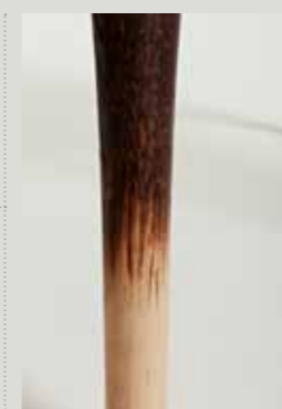
Legs were blackened with a blow torch - rather like spit roasting
