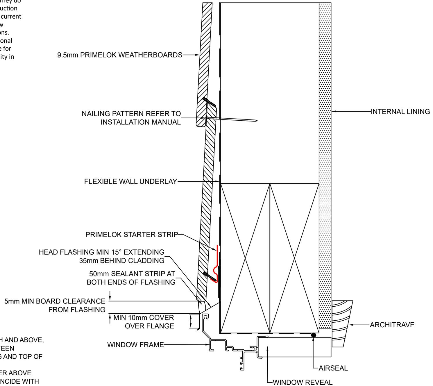
NOTE: IN WIND AREAS OF VERY HIGH AND ABOVE, SEALANT MUST BE INSTALLED BETWEEN UNDERSIDE OF THE HEAD FLASHING AND TOP OF THE WINDOW HEAD FLANGE
