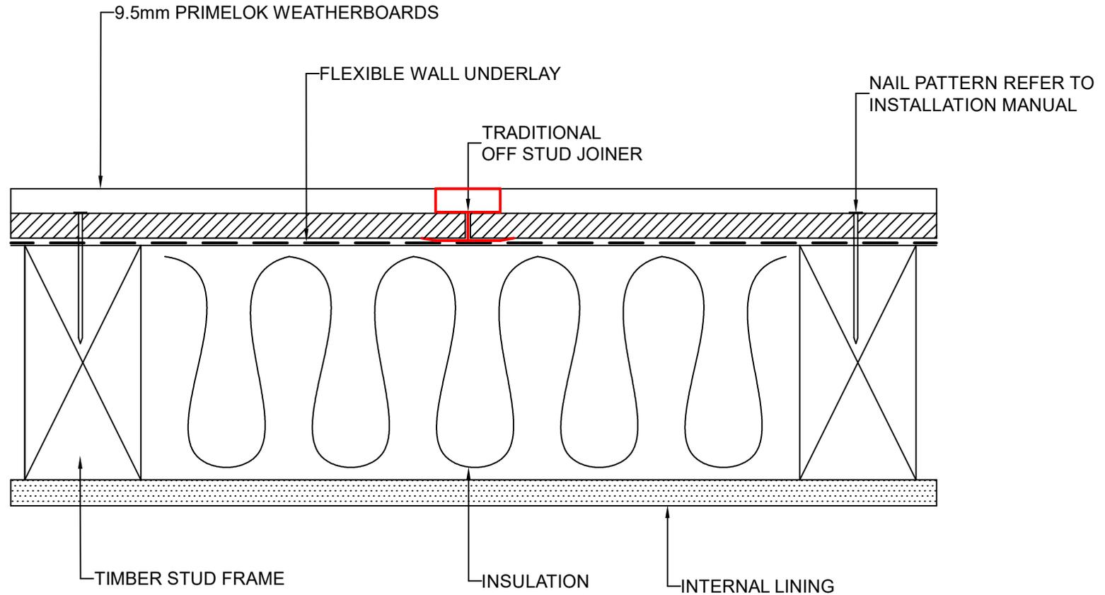
These drawings are for information only. They do not contain full details required for construction and must be used in conjunction with the current issue Weathertex Installation Manual, New Zealand Building Code and Local Regulations. Weathertex recommends gaining professional advice to ensure the drawings are suitable for your project. Weathertex accepts no liability in respect to the use of these drawings.
