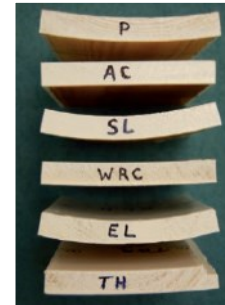
Accoya was the only wood that did not cup in this BM Trada trial. From top to bottom: Pine, Accoya Wood, Siberian Larch, Western Red Cedar, European Larch and Thermowood.
