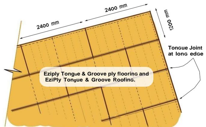
Maximum Spacing @ 400 mm Fixings @ maximum 150 mm to all edges and 300 mm to Central Joists
