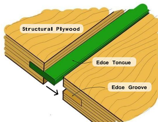
**Typical ITI Timspec Structural Plywood Tongue & Groove**
