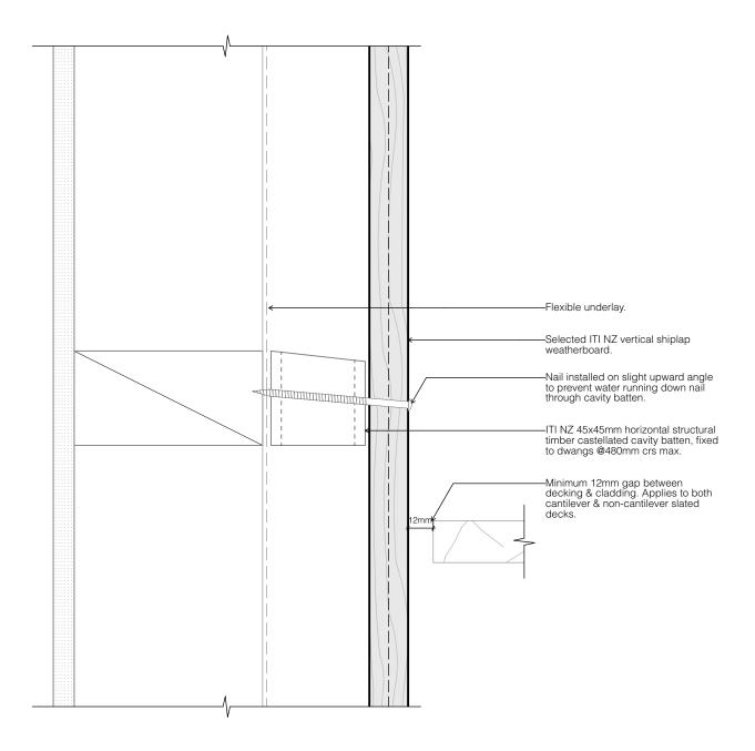
DETAIL 13.22 - 701 ROOF / WALL - FLAT SOFFIT
