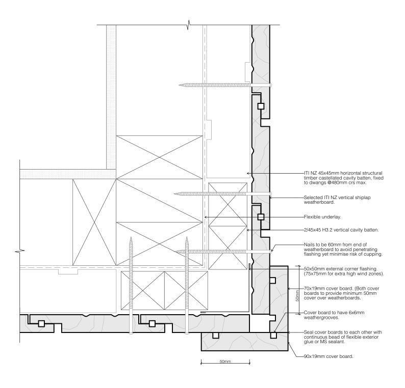
DETAIL 13.15 - 502 EXTERNAL CORNER - P42 CORNER MOULDING
