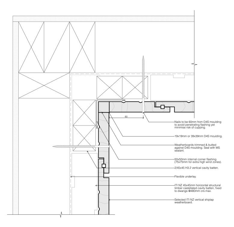
DETAIL 13.12 - 402 INTERNAL CORNER - 39X39MM INTERNAL MOULDING
