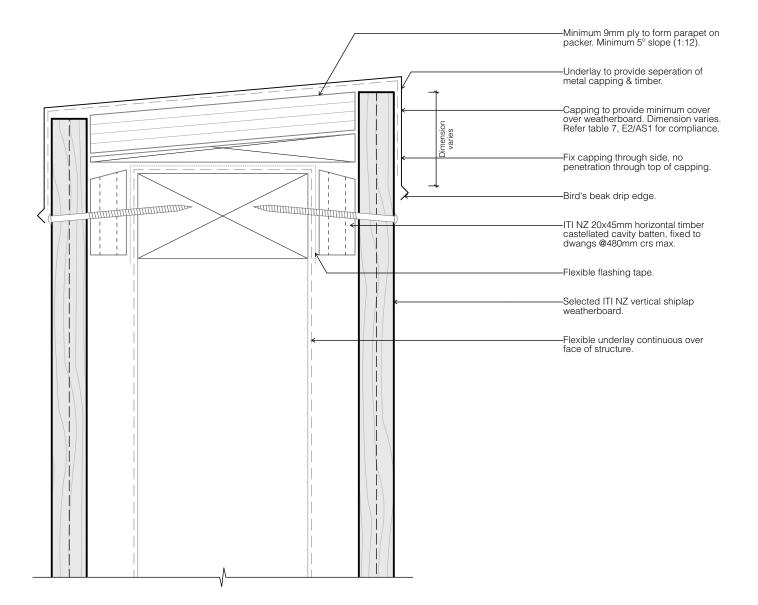
DETAIL 13.25 - 802 PARAPET - INTERSECTION WITH WALL
