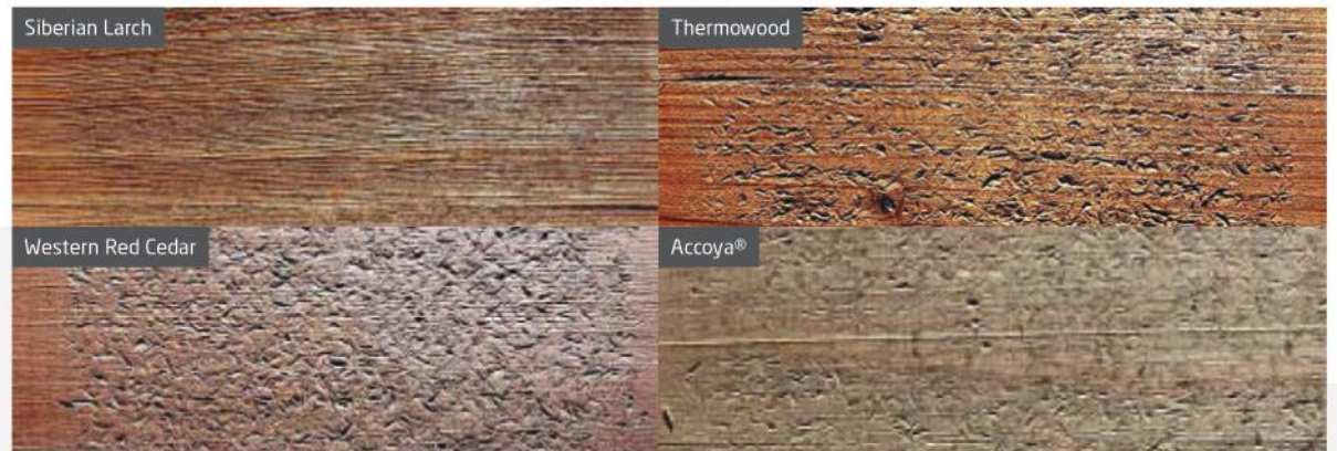
4 wood types compared for scuff resistance by the Snell Capsule Method at TRADA
