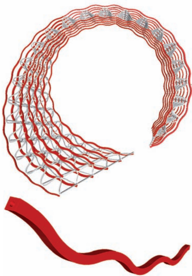
The 88 curved chord elements were built up from thin layers of glued laminated timber. There are 14 types of chord elements with a length range of 2,600mm to 4,600mm
