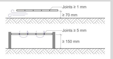
The subsurface the decking is installed on should be sufficient strong and rigid and with a slope of at least 2% (up to 5%). In case of an insulation layer beneath the deck, this material should have a sufficient high compressive strength.
