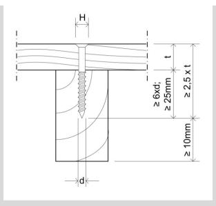
The recommended point side penetration of screws into the sub-frame is at least 25 mm, 6 x shank diameter or 1.5 x board thickness (whichever is the largest).
