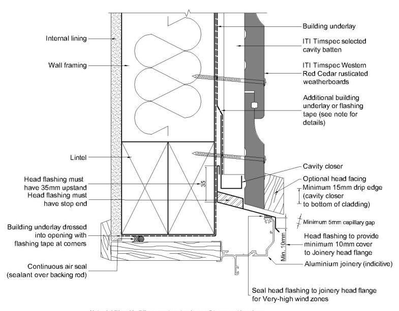
Note: Additional building wrap to extend up wall to nearest lap above and extend down as far as possible into cavity closer.
