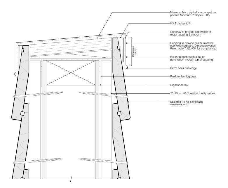
DETAIL 13.21 - 802 PARAPET - INTERSECTION WITH WALL
